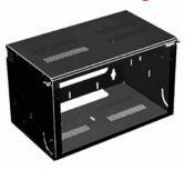
Hinged panel pivots to 90 degrees with positive stop, providing a stable platform for punch-down interconnects. Thumbscrews secure the panel in the upright position. Integral VELCRO® cable tiedown slots facilitate cable routing. Cover protects equipment and cables. Made of 12 gauge steel on hinged swing-out frame; 16 gauge on body. Finished with RAL 9005 low gloss black polyester powder paint. Shipped fully assembled.
